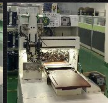
Auto soldering machine
