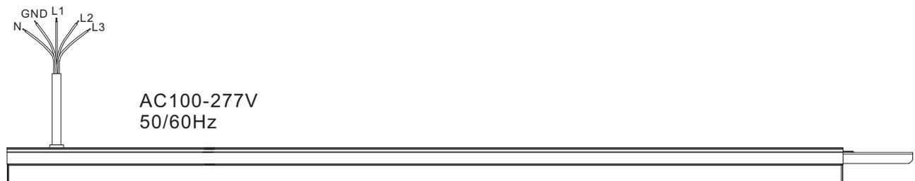
SL5550 non-dimming AC connection diagram
