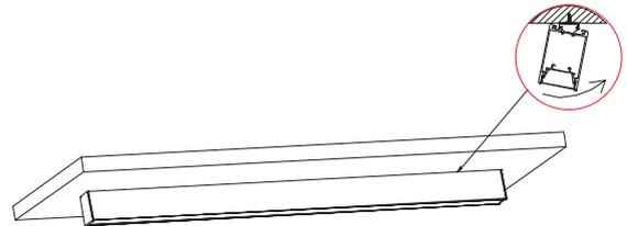
Step3:Thread 4X25PA screw through fixing hole of safety rope and clip, finally fix 4X25PA screw and rubber plug tightly.
